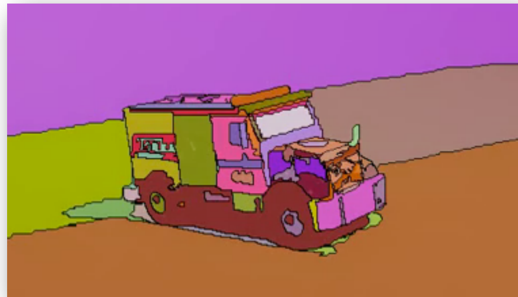
Hierarchical segmentation (shown at 50% of height of segmentation tree)
